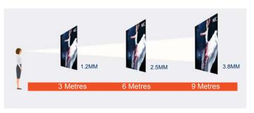
Pixel pitch is the distance from the centre of a pixel to the centre of any adjacent one. The smaller the pixel pitch, the higher the density and the clearer the image. Greater pixel density carries a higher price tag, so the best way to choose the right option is to consider the optimal viewing distance for the type of content - whether its text, images or video; and its application - whether for company presentations or for digital signage.
